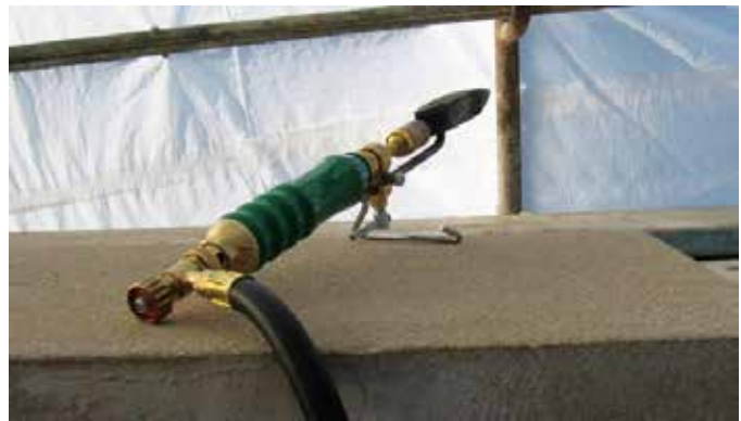
A commonly used soldering iron: copper-bit gas-fired soldering iron.
