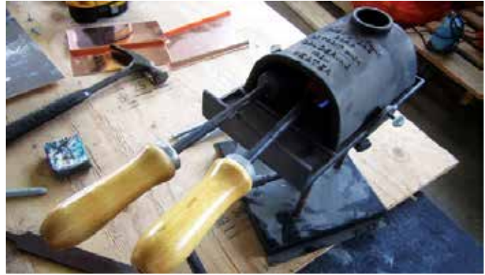
Commonly used soldering irons: hand coppers with propane pot.
